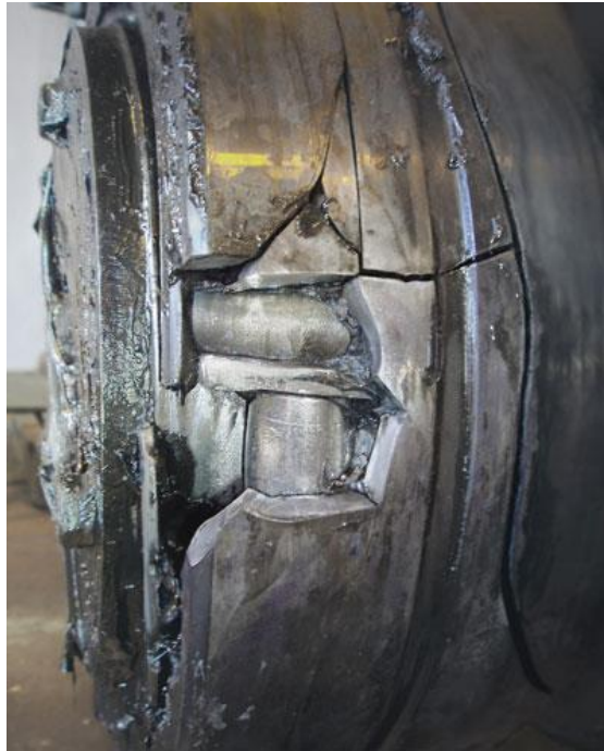
Large drum oven bearing with a crack detected using ultrasonic tools
